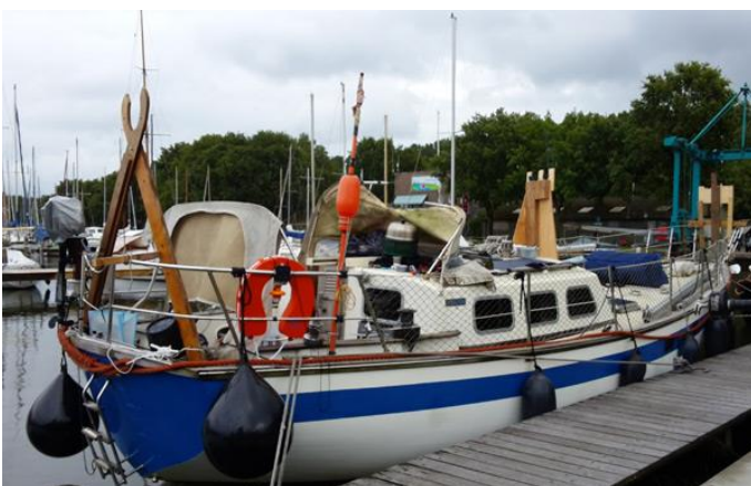
3 wooden structures aligned to carry the 2 masts
